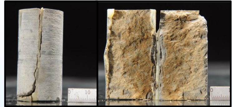
Fracture in Shaley Limestone
